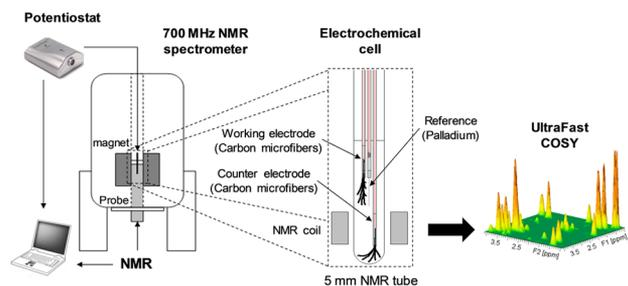
**Figure 1.** Schematization of an *in situ* EC-2D ultrafast NMR experiment.
