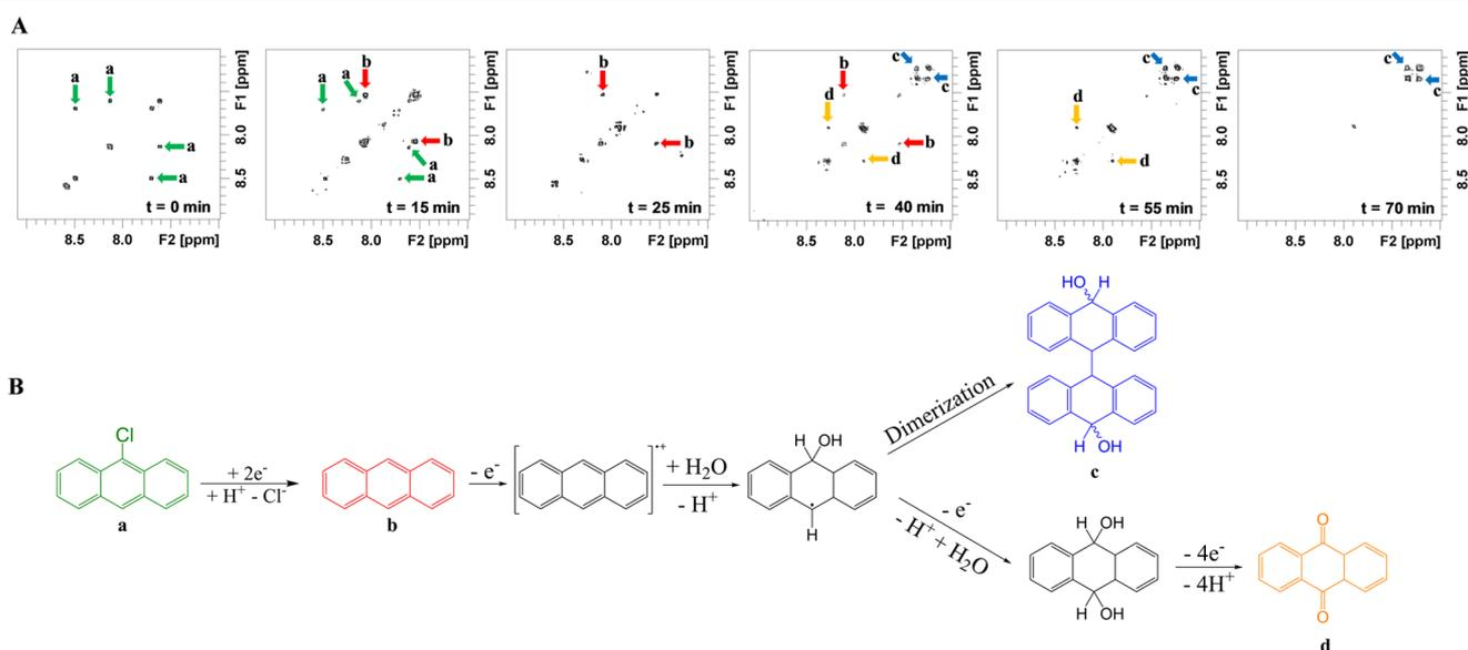
**Figure 2.** (A) Real-time 2D COSY NMR spectra recorded *in situ* during the electrochemical reduction of 9-chloroanthracene. The spectra were recorded in 3 min each, with the experimental setting of Figure 1. The correlation peaks of each compound are marked by arrows. Experimental details are given in the Supporting Information. (B) Redox behavior of 9-chloroanthracene based on these spectra.
