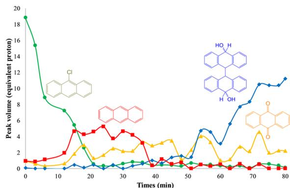
**Figure 3.** Evolution of the 2D peak volumes on COSY spectra recorded in real time during the electrochemical oxidation of 9-chloroanthracene, for the precursor (green circles), instable intermediate (red squares), and reaction products (blue rhombuses, orange triangles). For each compound, the volumes correspond to the average of the peaks marked by arrows in Figure 2, normalized to the number of equivalent protons.
