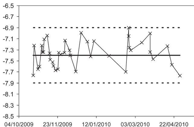
**Figure 1.** Quality control of the isotopic  $^{13}\text{C}$  NMR measurement: long-term reproducibility of  $\delta^{13}\text{C}_{\text{CH}_2}$  (‰) of the control ethanol, measured once per session to validate the session.
