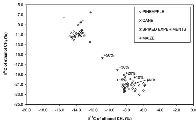
**Figure 3.** Two-dimensional plot of the site-specific  $^{13}C$  deviations of ethanol fermented from authentic pineapple juices, cane and maize sugars, and pineapple samples spiked with cane sugar (the percentages correspond to the proportion of added cane sugar in total sugars).
