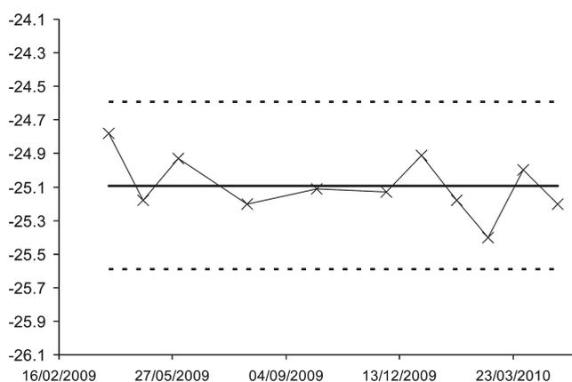
**Figure 2.** Quality control of the whole procedure (from the fermentation to the measurement): long-term reproducibility of  $\delta^{13}\text{C}_{\text{CH}_2}$  (‰) of the ethanol produced by fermentation of the sugars of a reference fruit juice, measured once per month.
