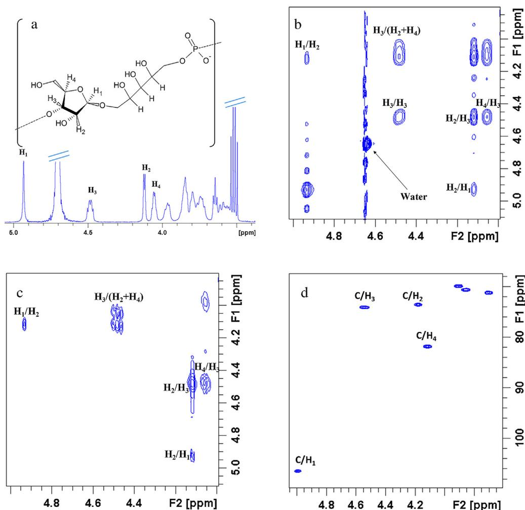
**Fig. 1.** Different NMR spectra of a 5.51 mmol L<sup>-1</sup> Poly(riboseyl-Ribitol-Phosphate) (PRP) sample in D<sub>2</sub>O, recorded at 500 MHz with a cryoprobe. (a) One-dimensional <sup>1</sup>H NMR spectrum and molecular structure of the PRP; (b) Two-dimensional ZQF-TOCSY spectrum; (c) Two-dimensional <sup>1</sup>H INADEQUATE spectrum; (d) Two-dimensional <sup>1</sup>H-<sup>13</sup>C HSQC spectrum.
