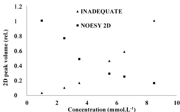
**Fig. 4.** Relative evolution of the sum of the 2D NOESY cross-peak volumes involving the  $H_2$  proton (normalized by the corresponding diagonal peak volume). For the sake of comparison, the evolution of the  $H_2/H_3$  peak volume for the  $^1H$  INADEQUATE experiment is also plotted. The data were obtained on a 500 MHz spectrometer equipped with a cryoprobe.
